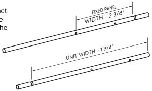
Level the Bar – Temporarily place the Wall Mount Sleeves [E] on each end of the Header Bar. Align the Header Bar with the Wall Mount. Place Block, and slide the Wall Mount Sleeves over the Wall Mount Blocks. a level on the center of the Header Bar and check for level. If needed the Wall Mount Blocks can be raised, or lowered to make the Header Bar level. Once leveled, remove the Header Bar from the Wall Mount Blocks, and the Wall Mount Sleeves from the Header Bar.
