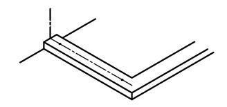
4 Channel Installation – Put a little silicone in the glass anchors. Then, install the Channel using the Screws [G] provided.
