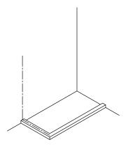
Mark the Wall Jamb Location – Place the SC-658 Wall Jamb [A] against the return wall with the holes lined up with the centerline marked in Step 1. Mark the center of all 3 holes on the centerline. Remove the wall jamb and drill all 3 locations for the Wall Anchors [C] you are using to mount the wall jamb. Clean the holes. Silicone, and insert the wall anchors, but do not install the wall jamb at this time.
