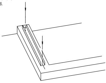
**5** Wall Jamb Installation – Mount the SC-658 Wall Jamb [A] to the return wall.
