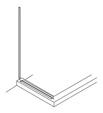
Return Panel Installation – Run a bead of silicone in the center of the the SC-658 Wall Jamb, and into the Bottom Channel. Then, orient the Glass Return Panel so that the return mount hole is toward the front of the enclosure. Slide the vertical edge of the glass into the siliconed SC-658 wall jamb. Set the bottom edge of the glass into the Siliconed Bottom Channel.
