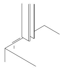
Return Channel Location - Place he Bottom Channel on the centerline. Mark the center of both nodes on the centerline. Remove the channel and dril both marks with 1/4" drill bit. Clean the holes and sill of debris, squirt a little silicone into the holes and insert the Glass Clip Anchors [D].
