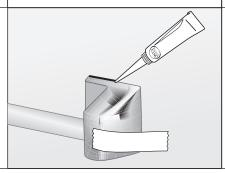
To smooth out a seamfill bead with your finger, dampen a paper towel with rubbing alcohol and then dampen your finger. Next, run your finger along the bead of seamfill, wiping any excess silicone onto the paper towel.
