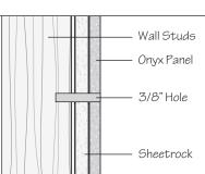
If the hole is tight, widen the hole slightly by running the drill bit in and out several times until the pin fits in smoothly.
