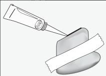
To smooth out a seamfill bead with your finger, dampen a paper towel with rubbing alcohol and then dampen your finger. Next, run your finger along the bead of seamfill, wiping any excess silicone onto the paper towel.
