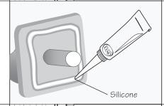
Leave about and 1/8" gap around the edge and the silicone so that it doesn't squeeze out when the shelf is pressed against the wall.
