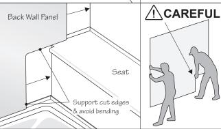
We recommend using two people to install this panel to avoid bending where panel has been notched. Carefully support the cut edges and guide into place as the panel is supported on the other end.
