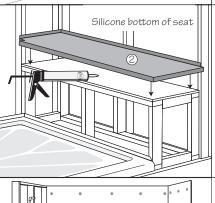
The bench seat should overhang the framing on the front and open side by 1" to 1 1/4" to accommodate the wall board and Onyx Panels. It is a good idea to frame the back of the bench 1/4" higher to allow for drainage.
