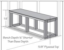
Walls should be plumb and framing should be completed before the shower base is installed. It is a good idea to make the back of the bench seat frame about 1/4" higher than the front so water will drain off the seat.
