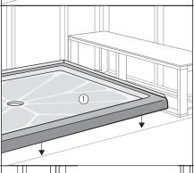
The base should extend ½"past the framing of the bench seat framing.
