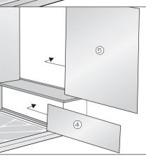
Seat front panel should come to the end of the base & will be capped by side panel
