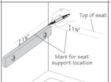
Installing the wood supports level will ensure correct drainage on the seat when installed.
