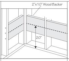
The 2" x 10" wood backer should be secured soundly to the wall studs.
