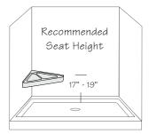
Using painter's tape on the shower wall to mark the location of the top of the seat will be helpful to maintain the correct height for marking the holes.
