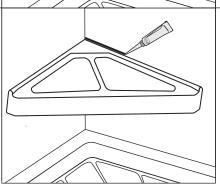
To smooth out a seamfill bead with your finger, dampen a paper towel with rubbing alcohol and then dampen your finger. Next, run your finger along the bead of seamfill, wiping any excess silicone onto the paper towel.
