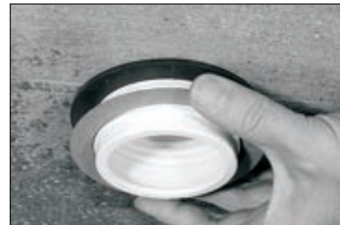
Rubber Washer First, Then Slip Washer
