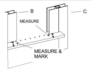
Slide bench curb (E) into bench wall jamb. Place black setting block (N) down inside of bench curb. Dry fit Bench glass. Glass should sit 1/8" from top of wall jamb (B). If every thing fits properly then remove glass. Fill bench curb track with silicone (this is called wet glazing). Place glass down into bench curb. Place transition post down inside curb track and down over top bench seat.
