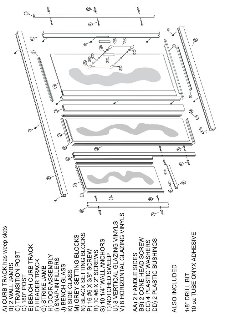
Your ONYX shower door is completely reversible and can be installed to swing left or to swing right. The door can also swing off of any post. For best waterproofing, The hinge side should be opposite the shower head. Use the illustration to determine where the hinge should be installed.
