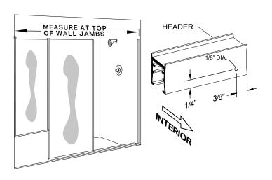
Place header track (F) over top of the all the jambs. Level all the center posts, then pre-drill 1/8" holes into the center posts (BE CAREFUL NOT TO DRILL THE GLASS BECAUSE IT WILL BREAK). Screw header track into place.
