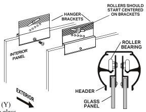
**CAUTION –** Do not over tighten the brackets and cause the end to clamp down on patterned glass. Do NOT use a screw gun. This can cause the glass panel to shatter.
