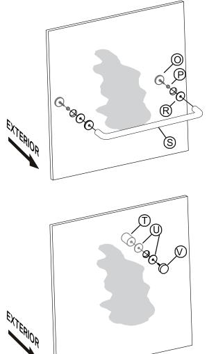
**B** Place plastic washer [U] on knob cap screw [V]. Place the knob cap screw [V] through the glass panel. Place other plastic washer [U] on knob cap screw [V]. Screw the knob [T] onto the knob cap screw [V].
