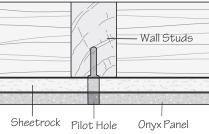
Screw the pointed end into the wall studs or wood backing so that 1" of the bolt remains protruding out from the wall. A good way to do this is to put the bolt in the end of a screw gun, this will help prevent damaging the threads.
