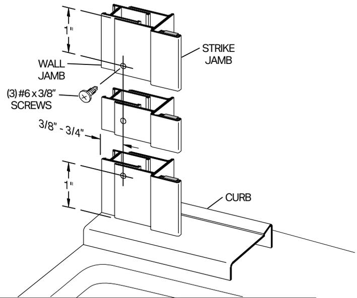
**6** Slide the hinge jamb of the door panel assembly [B] over the mounted wall jamb [C] so the door will open outward. Adjust the door panel assembly so there is 1/4" clearance between the strike jamb and the strike edge of the glass door panel in the closed position. Mark the location of the hinge jamb on the wall jamb with a pencil.
