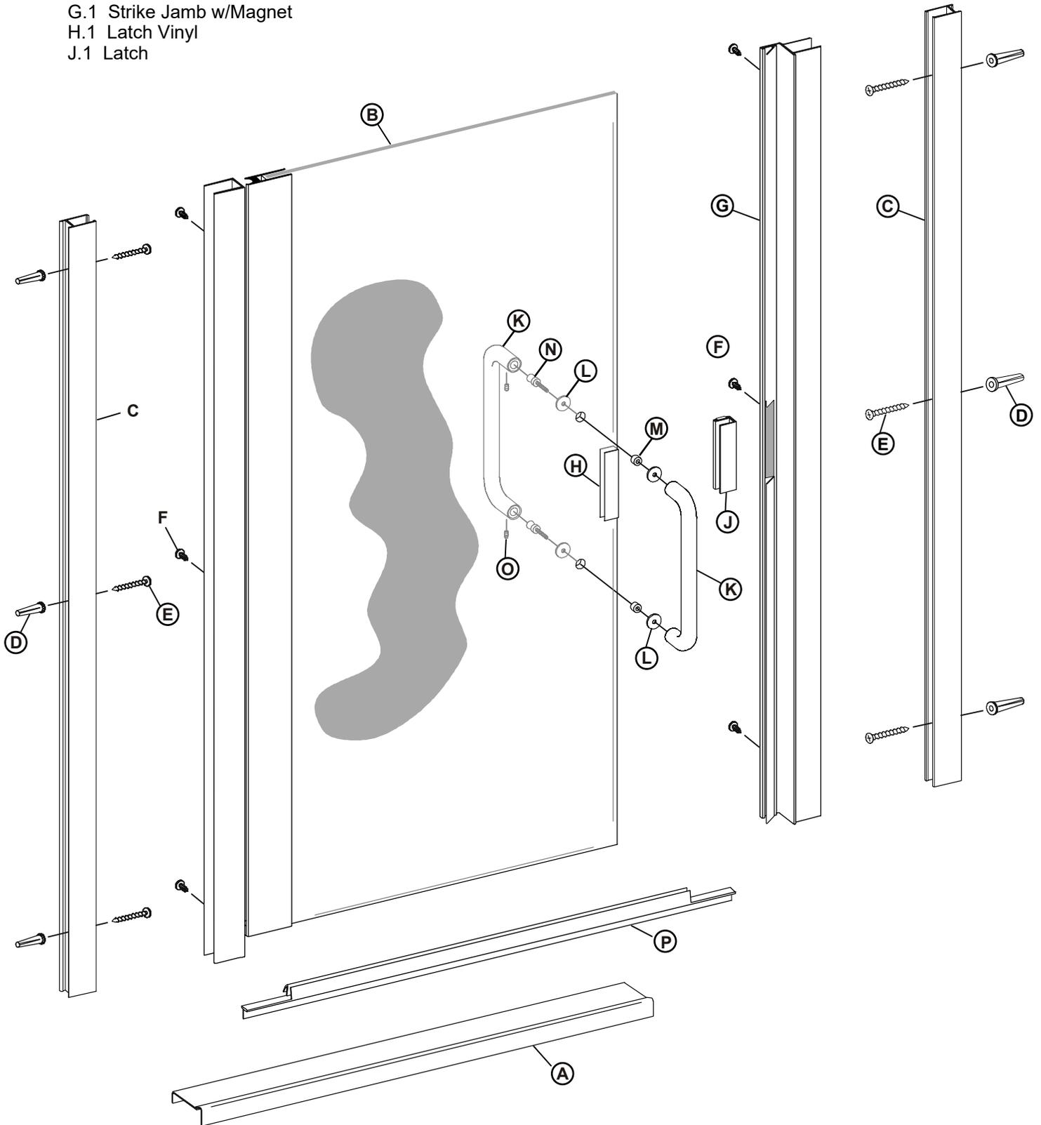
**1** Refer to the illustration to determine the correct position for your installation. For maximum waterproofing, the hinge jamb should always be opposite the shower head. These instructions depict a hinge-left and hinge-right installation based on shower head location.
